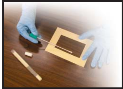
Surface Swab Kit contains 10 sterile swabs in transport tubes and 10 templates (5 x 10 cm)
